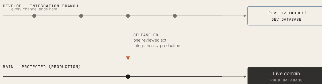
Figure 8 — One trunk, one reviewed release. Every change lands on develop , which continuously serves a development environment on its own database. Production is the protected main branch on a separate database and domain, advanced only by a single reviewed integration-to-production request. A release is a deliberate act.
